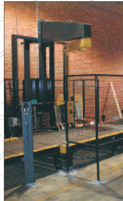
Automatic compression strapper used in wrap bulk, column stacked newspaper in
