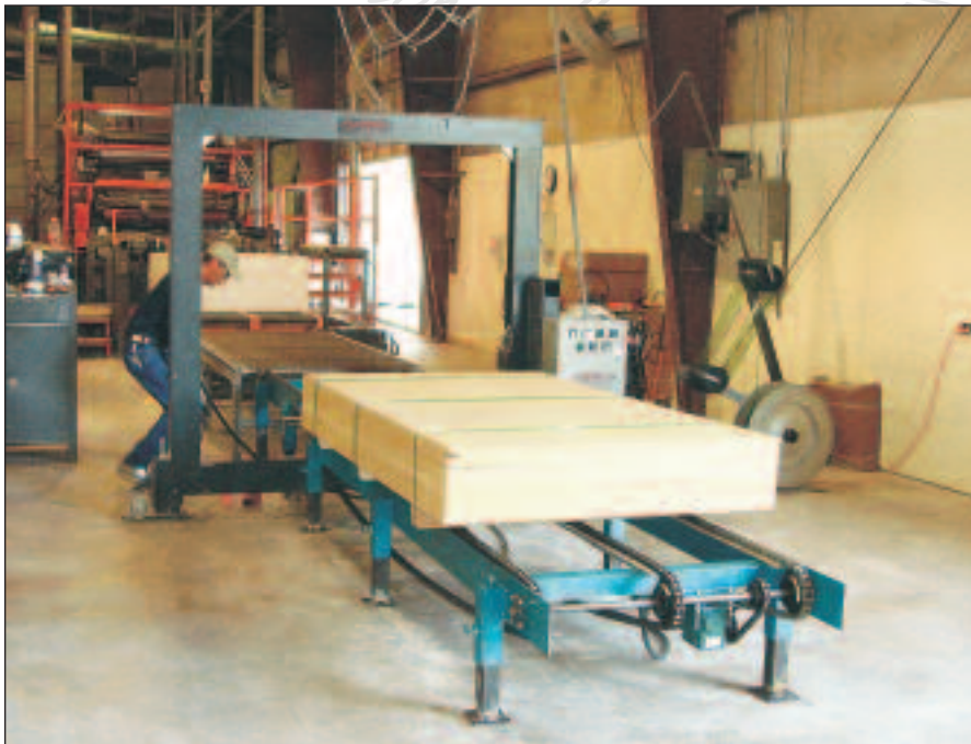
PAC installed system for sheetrock. System includes automatic strapper, conveyor and bunk applicator.
