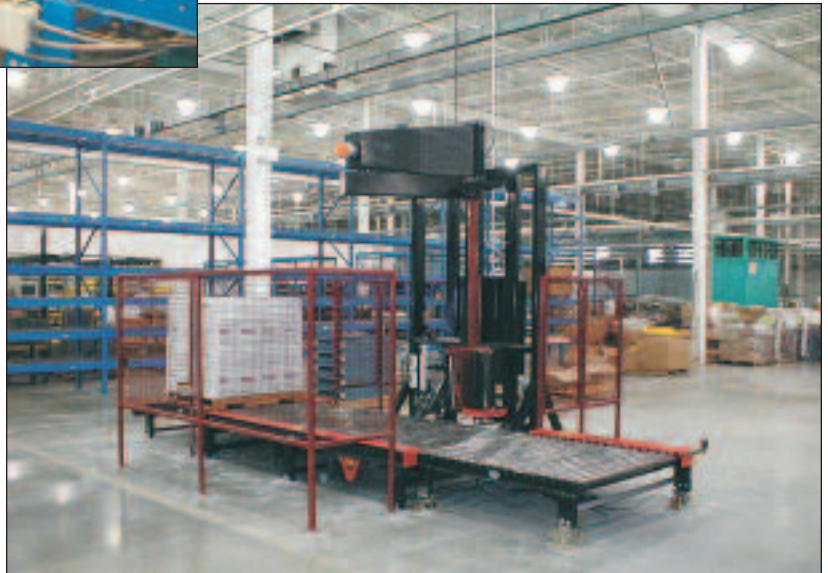
Typical PAC strapping system for boxed finished goods.
